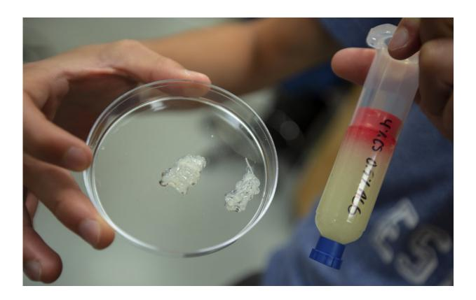
A pair of 3-D printed scaffolds made from bio-inks rest in a petri-dish. The bioink (right) used to create these structures is a mix of chitosan (a compound made from the shells of shrimp and other crustaceans) and alginate. Credit: Troy Fedderson/University Communication
