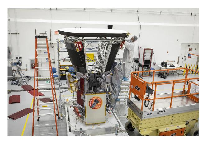
The Thermal Protection System connects to the custom-welded truss on the Parker Solar Probe spacecraft at six points to minimize heat conduction. Credit: NASA/Johns Hopkins APL/Ed Whitman
