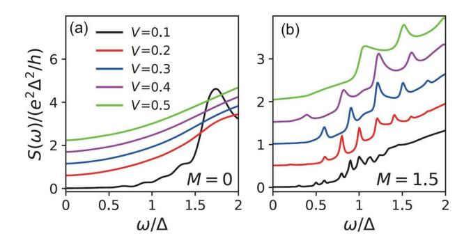
The non-equilibrium noise at a finite frequency for various values of the applied bias voltage for a topo-logical Josephson junction with two different transmission probabilities D = 1 (a) and D
