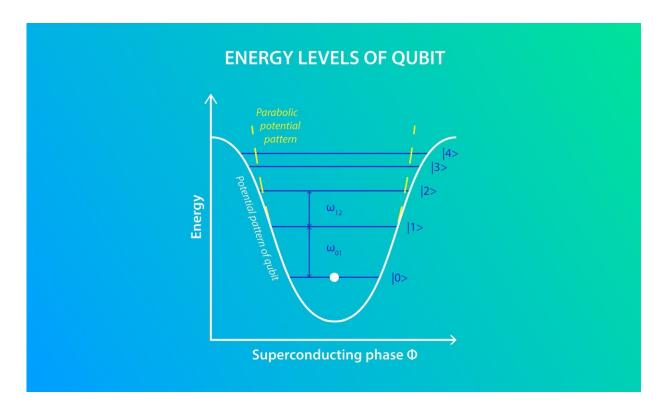
Figure 2. The energy spectrum of a transmon is similar to that of an atom. The frequency of the transition between the first two energy levels is  $\omega_{01}$ . Credit: Elena Khavina/MIPT
