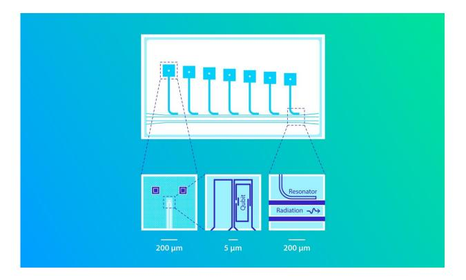
Figure 3. Microwave chip. Each of the seven square regions in the top picture contains a qubit. The L-shaped lines in the top picture are microwave resonators, each of which has a distinct resonant frequency. A micrometer  $(1 \mu m)$  is one-millionth of a meter. Credit: Elena Khavina/MIPT
