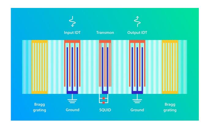
Figure 1. Schematic of the chip. The resonator is a Fabry-Perot cavity formed by two Bragg gratings, each consisting of 200 parallel stripes (shown in yellow) separated by half the acoustic wavelength. The wavelength is equal to 0.98 micrometers, or 980 nanometers. There are two interdigital transducer (IDT) ports — a receiver and a transmitter — and a qubit (transmon) inside the resonator. SQUID is the part of the transmon sensitive to weak magnetic fields. Credit: Elena Khavina/MIPT
