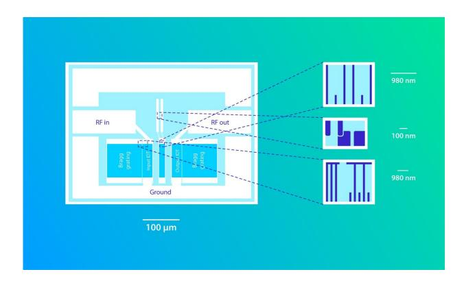
Figure 4. Acoustic chip. The size of the entire system is comparable to that of the magnified square region in figure 3. A nanometer (1 nm) is one-billionth of a meter and one-thousandth of a micrometer (1  $\mu$ m). RF stands for radio frequency. Credit: Elena Khavina/MIPT
