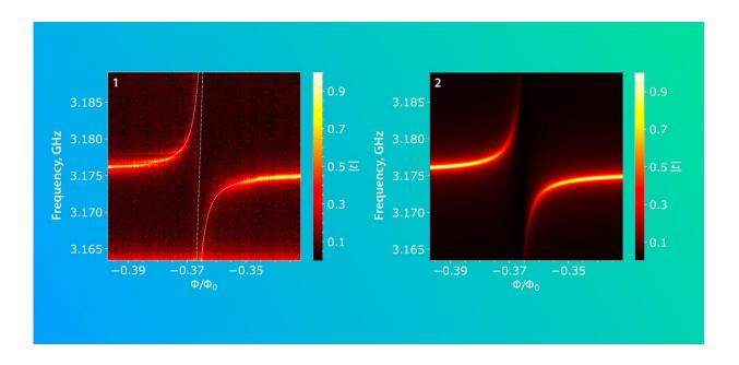
Figure 5. The intensity of the signal transmitted through the resonator is color-coded as a function of signal frequency and the magnetic flux. The experimental measurements are shown in (a) next to the theoretical predictions (b) based on the solution of the quantum model equation. Credit: Elena Khavina/MIPT
