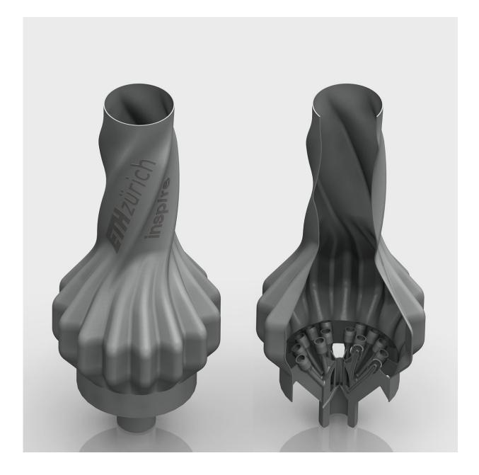
The burner is rippled to increase its surface area; the complex interior structures enable efficient air and gas supply to the combustion chamber. Credit: ETH Zurich / Patrick Beutler
