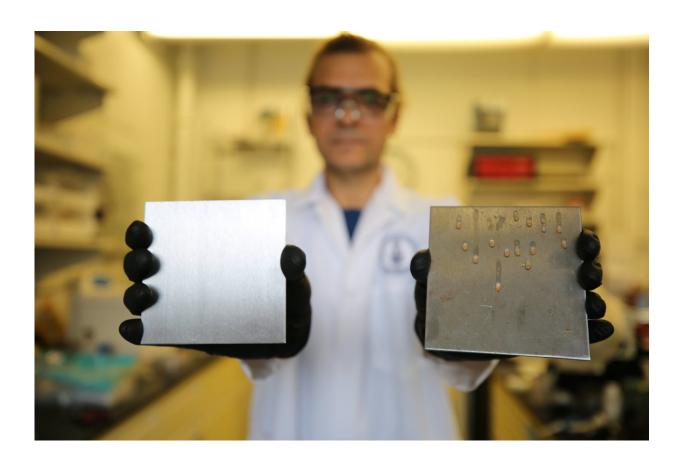
Dr. Tarek Awad, a researcher in the University of Toronto's Department of Materials Science & Engineering, shows two samples: at left, a stainless steel surface treated to trap simple cooking oil, and at right, an uncoated surface. The uncoated surface can accumulate food residue and encourage the growth of foodborne pathogens. Credit: Liz Do
