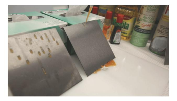
Food particles can accumulate on an untreated stainless steel surface, at left, increasing the risk of contamination in food production facilities. The oil-treated surface, at right, repels material. Credit: Liz Do
