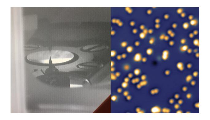
LEFT: STM image of Holmium single atom magnets. RIGHT: and Cobalt helper atoms on magnesium oxide. Credit: F. Natterer/EPFL
