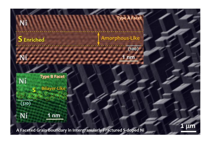
Faceted grain boundary in intergranularly-fractured sulfur-doped nickel. Credit: Jian Luo et al.
