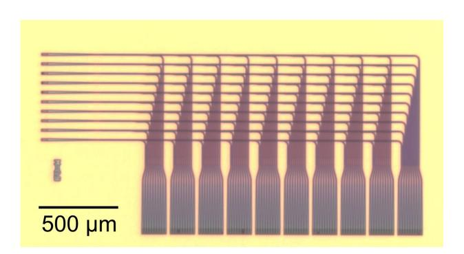
NIST's grid-on-a-chip distributes light signals precisely, showcasing a potential new design for neural networks. The three-dimensional structure enables complex routing scheme, which are necessary to mimic the brain. Light could travel farther and faster than electrical signals. Credit: Chiles/NIST
