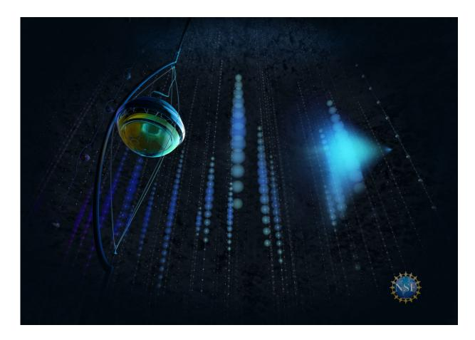
When a neutrino interacts in the clear Antarctic ice, it produces secondary particles that leave a trace of blue light as they travel through NSF's IceCube detector. Credit: Nicolle R. Fuller/NSF/IceCube
