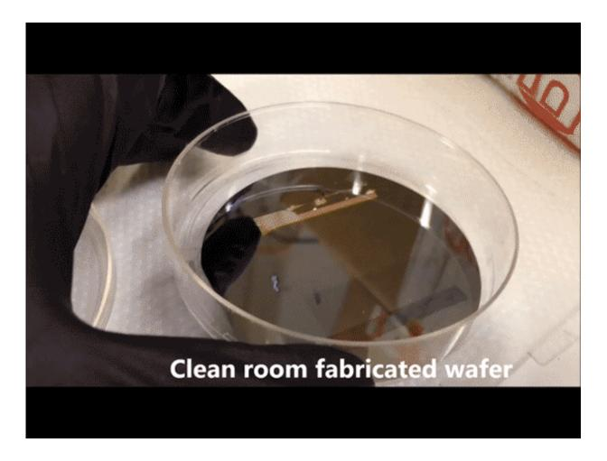
Researchers produced tiny electronic circuits, just 100 micrometers across, on a substrate material which was then dissolved away to leave the individual devices floating freely in solution. These were later attached to tiny colloidal particles. Credit: Massachusetts Institute of Technology
