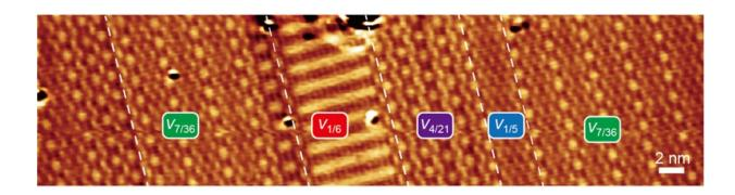
Scanning electron microscope images reveal a borophene sheet containing domains with different periodic assemblies of known hexagon-to-triangle ratios of 1-to-5 and 1-to-6 rows, along with two previously unobserved phases of 7-to-36 and 4-to-21. Scientists at Rice and Northwestern universities made the first detailed analysis of ordered defect structures in borophene. Credit: Hersam Research Group/Northwestern University
