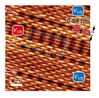
Scanning tunneling electron microscope images of line defects in 1-to-6 and
