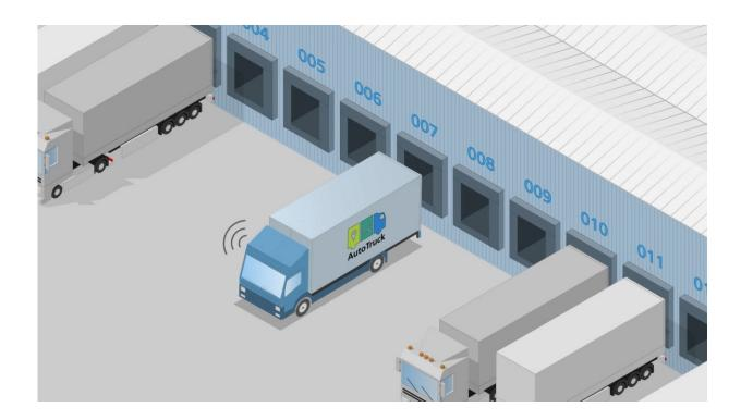
The truck drives independently to the loading ramp and waits until it is loaded. Credit: Fraunhofer IVI
