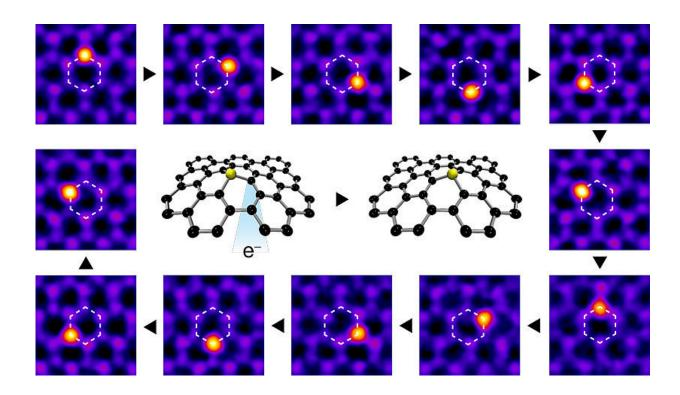
An electron beam focused on a carbon atom next to a silicon impurity atom can controllably make it jump to where the beam was placed. Step by step this allows the silicon to be moved with atomic precision around a hexagonal path. Credit: Toma Susi / University of Vienna
