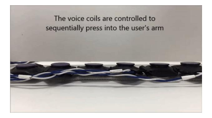
Tiny speakers, or voice coil actuators, embedded in the armband rise and fall to mimic the sensation of a human touch. Credit: Video/Heather Culbertson
