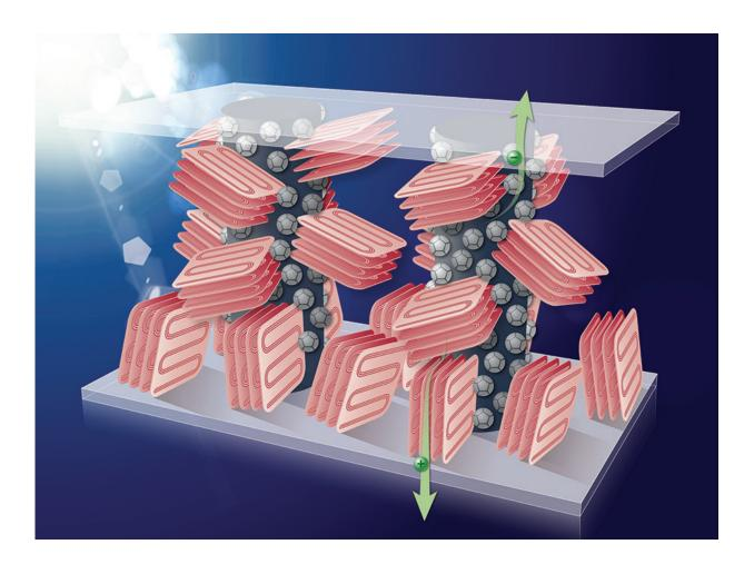
Adding an inert polymer component in plastic solar cells – as visualized by the arrows in this image -- creates a unique columnar morphology and enables increased optimal device thickness, which is much better suited for the industrial production of solar cells by low-cost solution coating methods. Credit: Stony Brook University
