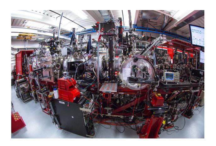
The experiment was performed at the Coherent X-ray Imaging (CXI) instrument, which makes use of the rapid, brilliant X-ray pulses from the Linac Coherent Light Source. CXI applies the "diffraction-before-destruction" method to take measurements with ultrashort X-ray pulses before they damage their targets. Credit: SLAC National Accelerator Laboratory
