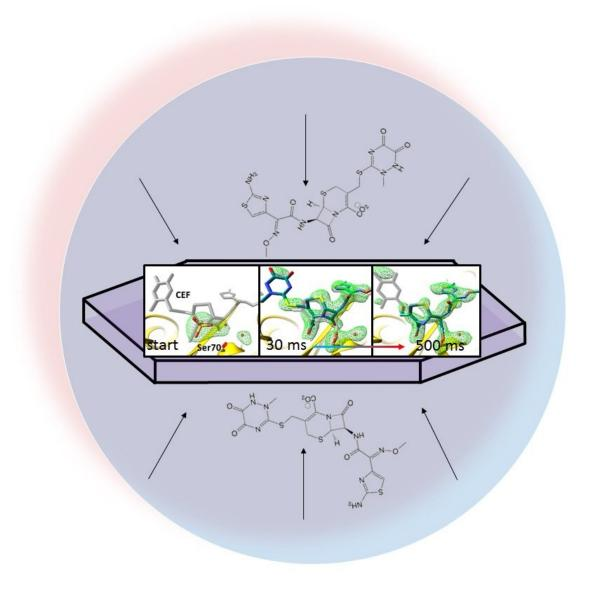
In a liquid droplet (represented by the light blue circle), an antibiotic disperses through a crystallized protein, beta-lactamase, and binds to it. X-ray snapshots of the bound pair allowed researchers to create maps of the electron density (green) and watch a ring in the antibiotic break open (far right) 30 to 500 milliseconds after the reaction began. Credit: Marius Schmidt / University of Wisconsin Milwaukee
