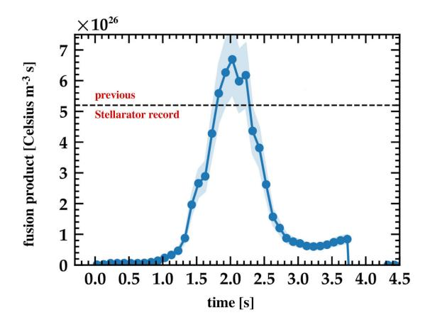
Wendelstein 7-X attained the Stellarator world record for the fusion product. This product of the ion temperature, plasma density and energy confinement time specifies how close one is getting to the power plant values needed to ignite a plasma. Credit: Graphic: IPP
