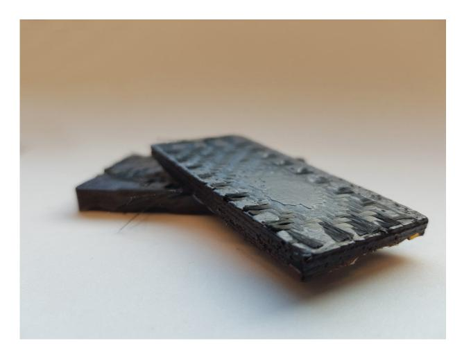
Carbon fibre mats can be used with the new epoxy resin. Credit: Vienna University of Technology
