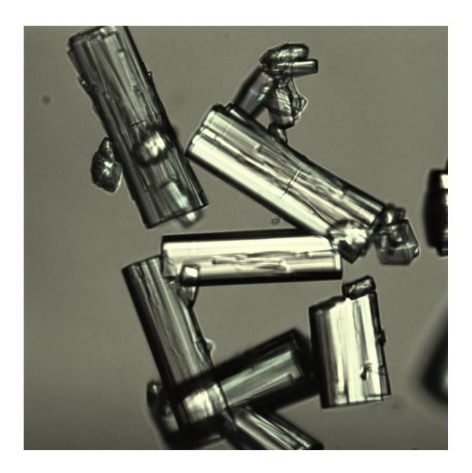
Optical microscope images of crystals of the newest, aluminum-based metalorganic framework, MOF-303, which captures twice as much water as the earlier MOF used in the water harvester Credit: Omar Yaghi laboratory, UC Berkeley
