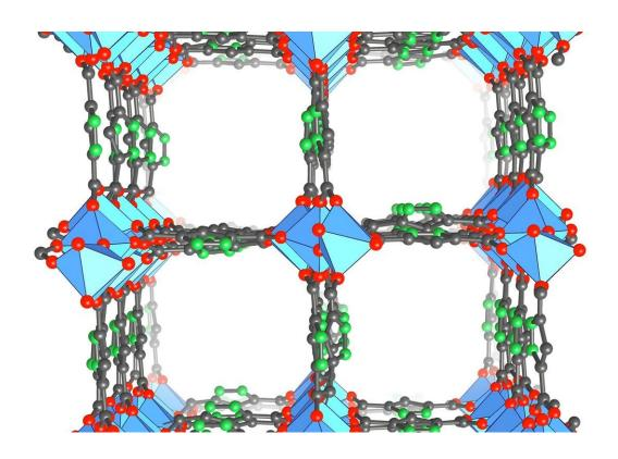
The crystal structure of the newest, aluminum-based metal-organic framework, MOF-303, which captures twice as much water as the earlier MOF used in the water harvester. Credit: Yaghi lab, UC Berkeley
