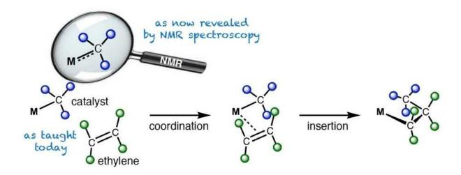
Polymerization of ethylene with organometallic catalysts (the M stands for the metal, typically Ti, Zr or Hf) as discussed in textbooks (bottom). The magnifying glass above illustrates the new findings revealed by NMR spectroscopy: the metal-carbon bond has a double bond character. Credit: Christopher Gordon / ETH Zürich
