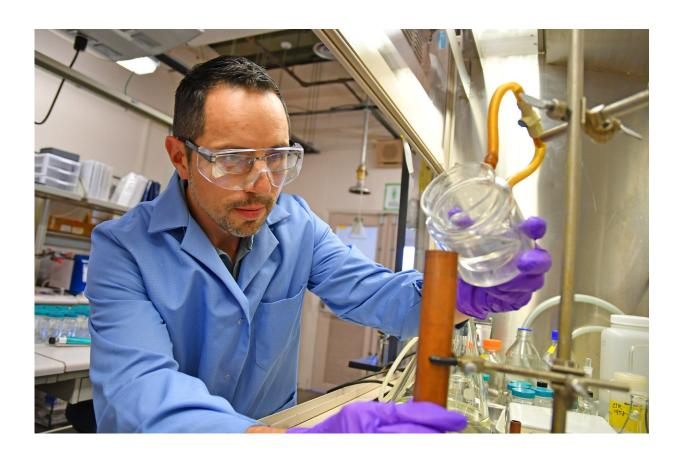
Explosives chemist David Chavez pours an example of melt-castable explosive into a copper mold at Los Alamos National Laboratory's Technical Area 9. Credit: LANL
