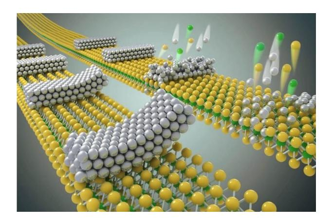
The new technique (left, foreground) prevents tiny defects from forming by laminating a thin sheet of metal (silver spheres) to the semiconductor layer (yellow), creating a better fit than the current process (right, background). Credit: University of California, Los Angeles
