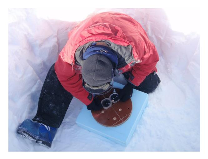
One of the researchers orienting a seismic censor after it was installed as a part of the array in East Antarctica. Credit: Amanda Lough
