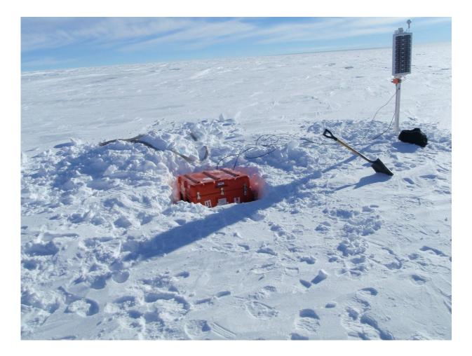
Installation of one of the monitors in the East Antarctica seismic array. Credit: Amanda Lough
