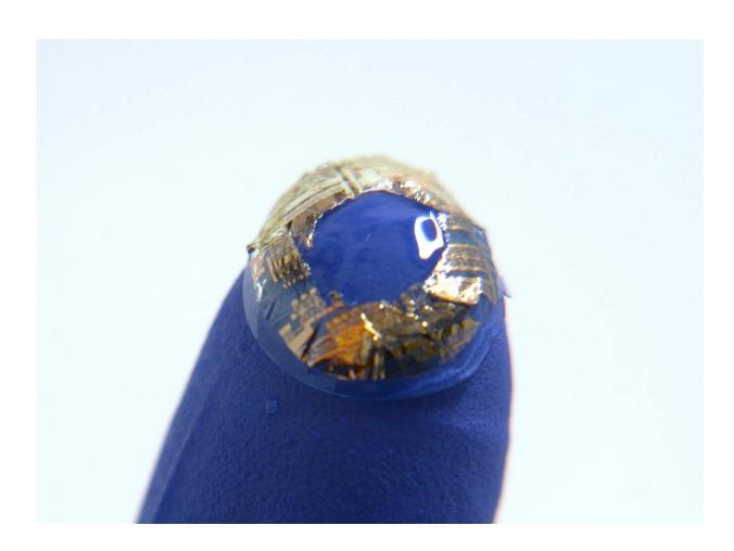
Purdue University researchers combined a commercial soft contact lens with an ultrathin conformal sensor circuit. Credit: Purdue University
