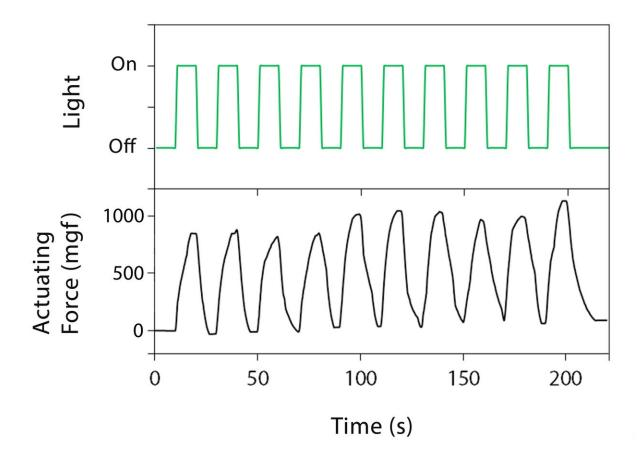
Figure 1 Actuating force of a 0.3-mg nickel hydroxide-oxyhydroxide actuator of under periodic light can reach about 1000-mg. Credit: The University of Hong Kong
