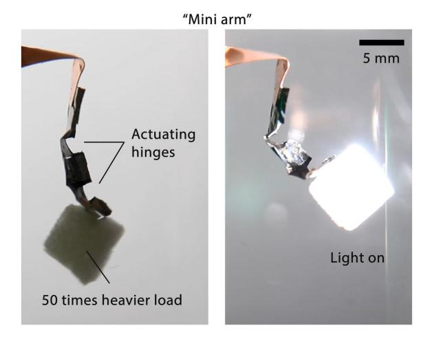
Figure 2. A mini arm with two actuating hinges lifting a weight 50 time heavier than itself under light. Credit: The University of Hong Kong
