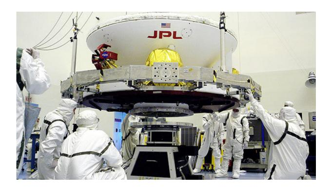
Engineers work on Opportunity (in its cruise configuration) in a cleanroom at Kennedy Space Center. A very important part of planetary protection is keeping contaminants from humans from riding aboard spacecraft. The pictured engineers are donning "bunny suits" that only allow their eyes to be exposed.
