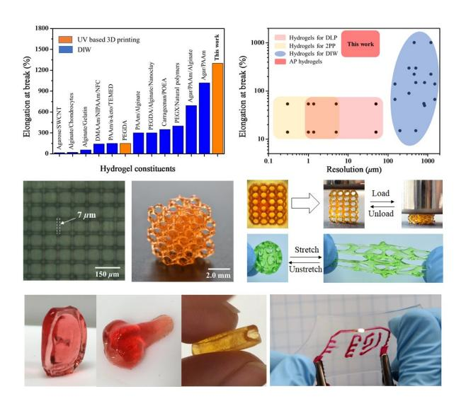
Highly stretchable and UV curable 3D printing hydrogels that can be stretched by up to 1300% and are compatible with high resolution digital light processing
