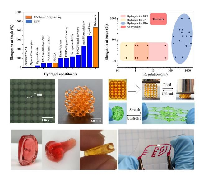
Highly stretchable and UV curable 3D printing hydrogels that can be stretched by up to 1300% and are compatible with high resolution digital light processing
