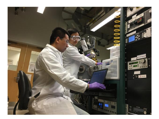
In this photo, Qiang Li makes a deposition program on the operational computer, and Yifan Zhang loads samples into a sputtering chamber to prepare highstrength Al alloy coatings. Credit: Purdue University
