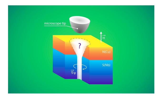
3-D graphic representation of the experiment using a scanning tunneling microscope: H denotes the external magnetic field whose direction is marked by the arrow,  $\phi$  is the phase of the superconducting wave function, and the interrogation point marks the area that was examined. Credit: Dimitri Roditchev, ESPCI-Paris, PSL University
