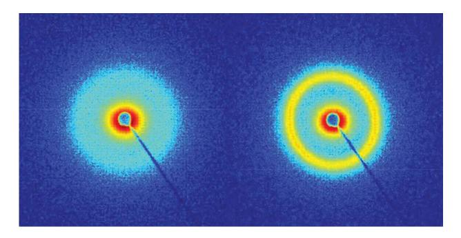
UD Professor Thomas H. Epps, III, suspected that lignin could be used to make adhesives with similar strength, toughness, and scratch resistance to the petroleum-based versions. These figures from small-angle X-ray scattering experiments show how a polymer created by Epps (left) compared with a commercial one. Credit: University of Delaware
