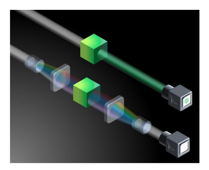
A broadband wave illuminates an object, which reflects green light in the shown example, making the object detectable by an observer monitoring the wave. A spectral invisibility cloak transforms the blocked color (green) into other colors of the wave's spectrum. The wave propagates unaltered through the object,
