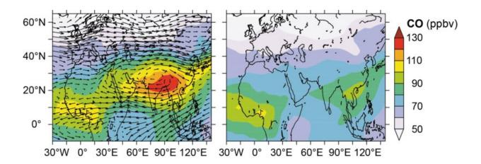
Modelling results illustrate atmospheric pollution over South Asia. The left figure shows carbon monoxide emissions (CO) at an altitude of 12 to 17 kilometres, on the right is the same visualization but without emissions from South Asia. The figure on the left also shows the winds over the region, clearly revealing the anticyclone created by the monsoon. Credit: MPI for Chemistry
