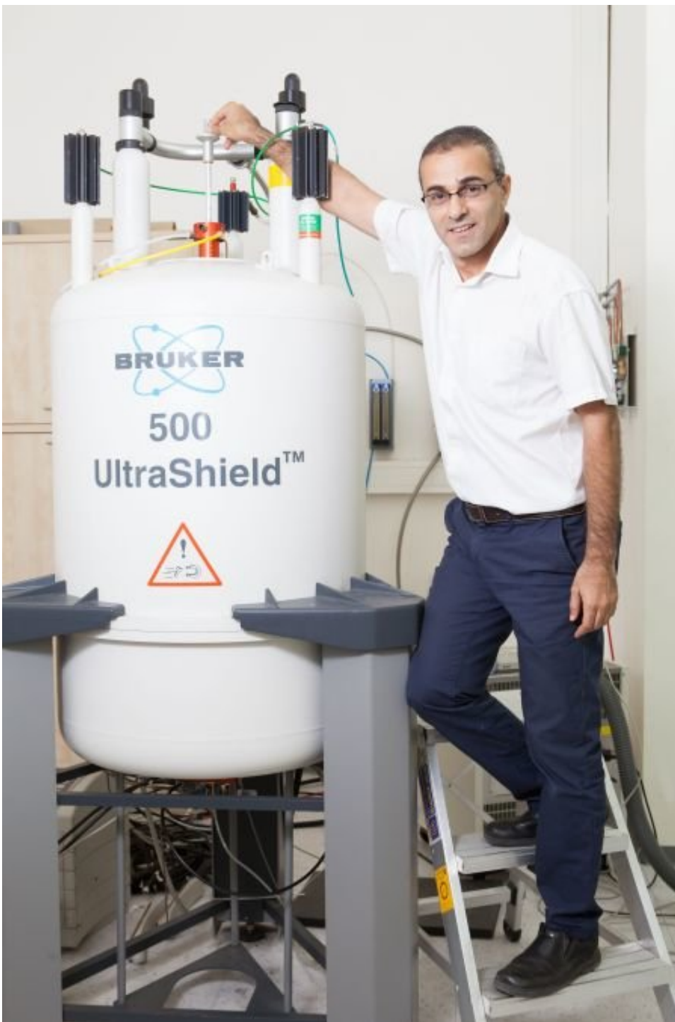
Prof. Gil Goobes, of the Department of Chemistry, standing by an 11.74 Tesla Bruker Avance III Spectrometer used for the solid state NMR experiments that were performed in the study. Credit: Bar-Ilan University
