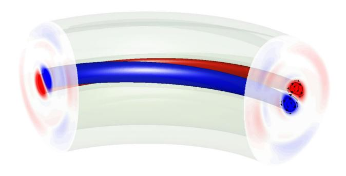
Helical plasma flow in the core of a tokamak in a nonlinear simulation. Red depicts positive values and blue depicts negative values of the poloidal velocity stream function. The black arrows illustrate the direction of the plasma flow within a toroidal cross section. (Figure shows a quarter of the torus.) Credit: US Department of Energy
