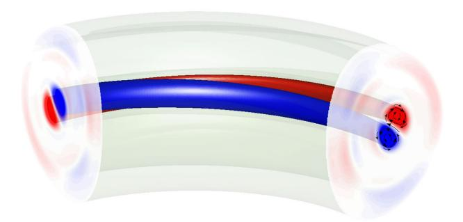
Helical plasma flow in the core of a tokamak in a nonlinear simulation. Red depicts positive values and blue depicts negative values of the poloidal velocity stream function. The black arrows illustrate the direction of the plasma flow within a toroidal cross section. (Figure shows a quarter of the torus.) Credit: US Department of Energy
