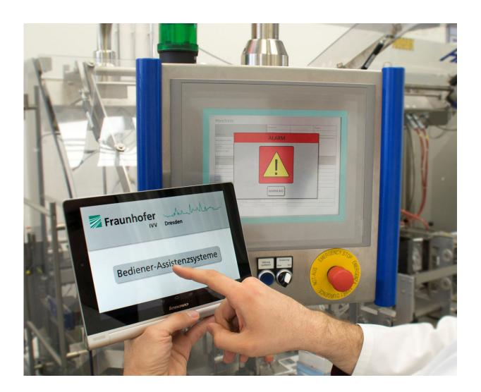
SAM, a self-learning assistance system, helps machine operators resolve errors in production machines. Credit: Fraunhofer IVV
