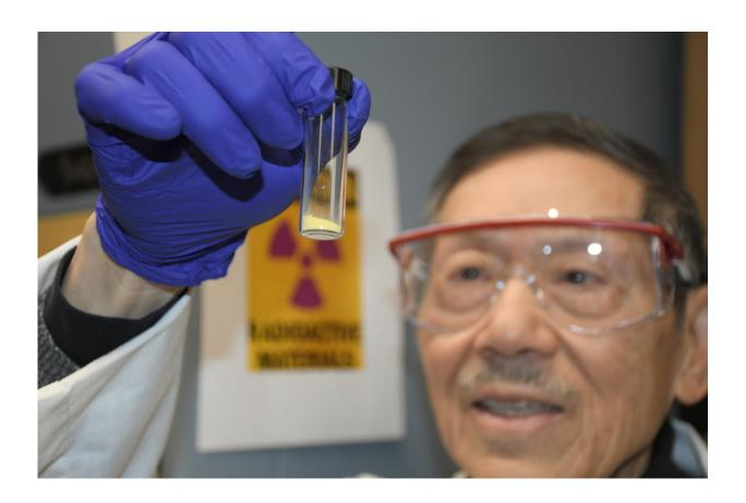
This first gram of yellowcake was produced from uranium captured from seawater with modified yarn. Chien Wai and colleagues at LCW Supercritical Technologies produced the yellowcake, a powdered form of uranium used to produce fuel for nuclear power production. Credit: LCW Supercritical Technologies
