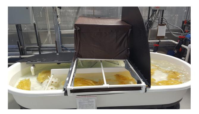
Material designed to capture uranium from seawater as an alternative to landbased mining of the fuel for nuclear power production is tested at PNNL's Marine Sciences Laboratory. Credit: PNNL
