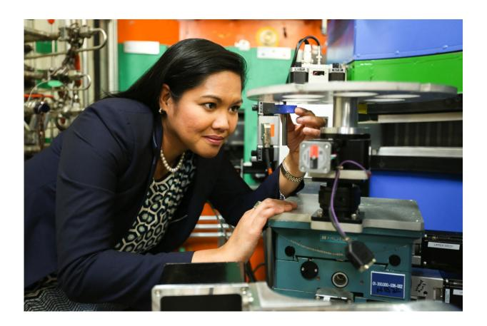
ORNL Instrument Scientist Clarina de la Cruz used the HB-2A Neutron Powder Diffractometer at the High Flux Isotope Reactor to analyze a cobalt-doped thermoelectric material boasting a record increase in room-temperature performance. Credit: ORNL/Genevieve Martin
