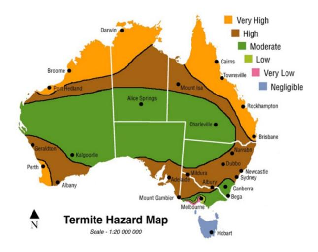
Figure 3. Termite infestation zones in Australia. Credit: termitesonline.com.au, Author provided
