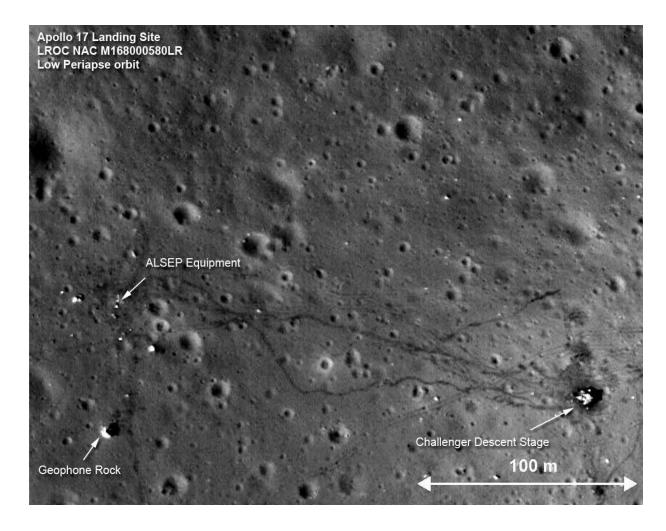
A Lunar Reconnaissance Orbiter Camera (LROC) image of the vicinity of the Apollo 17 landing site. Note the surface around the lunar surface experiment deployment site is darker than the surroundings. Credit: NASA
