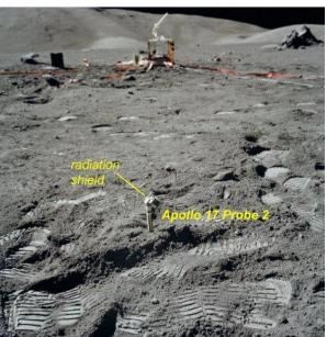
Left: This photograph by astronaut James Irwin shows the borestem and the cable of the Apollo 15 heat flow probe 1 protruding from the ground. Around the borestem, footprints of the astronauts can be seen. Right: This photograph by astronaut Harrison Schmidt shows the borestem and the cable of the Apollo 17 Probe 2 protruding from the ground. Credit: NASA
