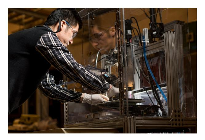
Ying Zhu, a developer of the nanoPOTS technology, places a chip containing samples for analysis into the automated system. Credit: Andrea Starr/PNNL
