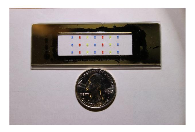
The chip containing multiple wells where proteins from single cells are separated out for further analysis. Credit: PNNL
