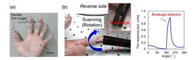
(a) Resting on a fingertip, the CNT THz imager can easily wrap around curved surfaces. (b) Just by inserting and rotating a flexible THz imager attached to the fingertip, damage to a pipe was clearly detected. Credit: *ACS Applied Nano Materials*
