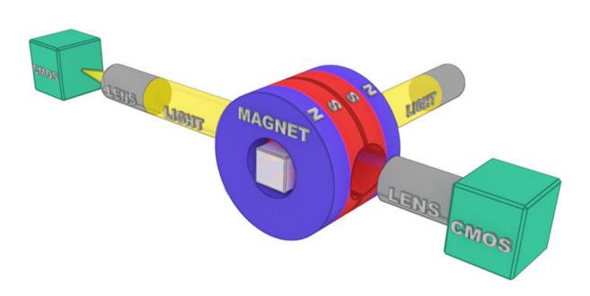
Schematic image of an experimental setup with a "magnetic well" trap for holding bio-objects. Credit: Vladislav A Parfenov et al // Biofabrication, 2018
