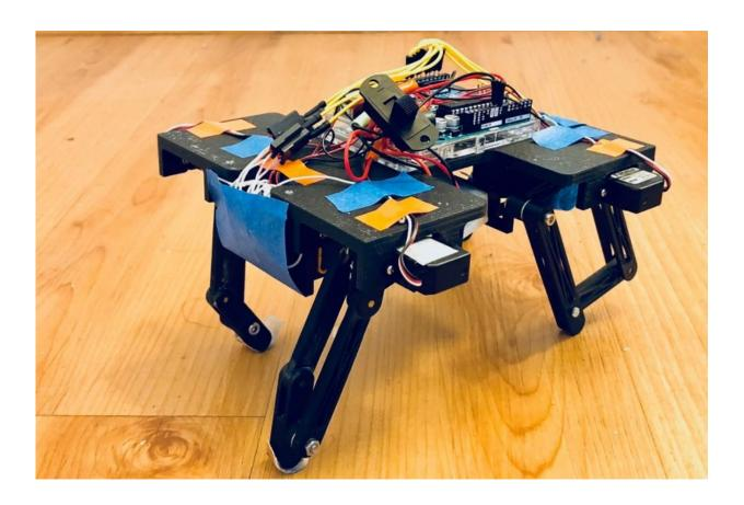
A four-legged robot was inspired by the motion of a cat. Credit: Photo/Daiming Yang
