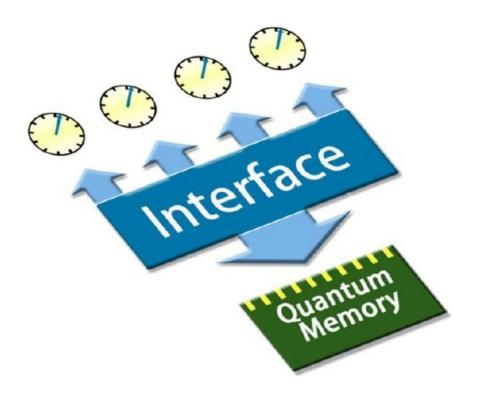
The quantum stopwatch transfers time information from a quantum clock, consisting of several identical particles, to a quantum memory. Credit: Yang et al. ©2018 The Royal Society
