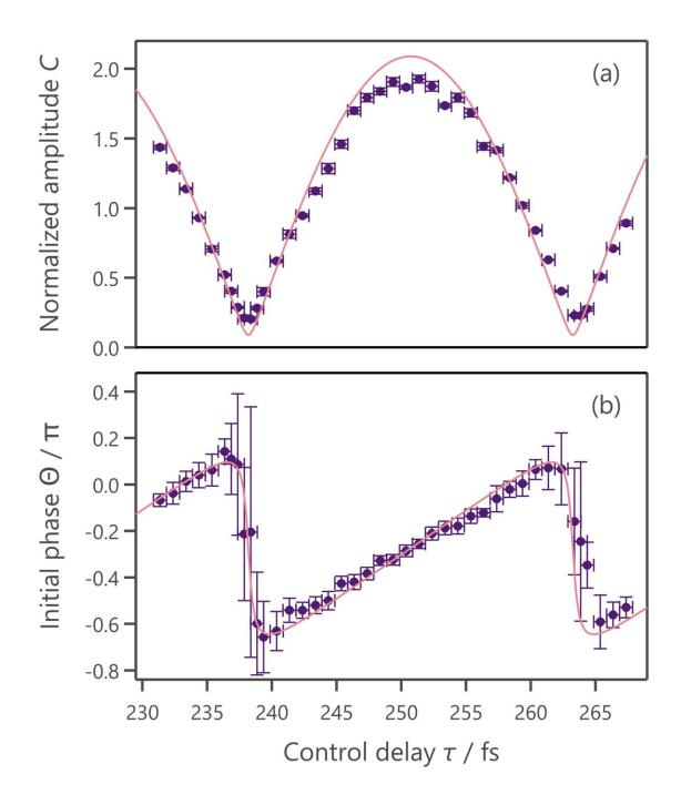
The points in the two figures show the experimentally measured amplitude (a) and phase (b) of the phonon oscillation with respect to the time gap between the two pump pulses. The points are consistent with the solid lines in the two figures, which represent the predictions of the proposed theory. Credit: Kazutaka.G.Nakamura
