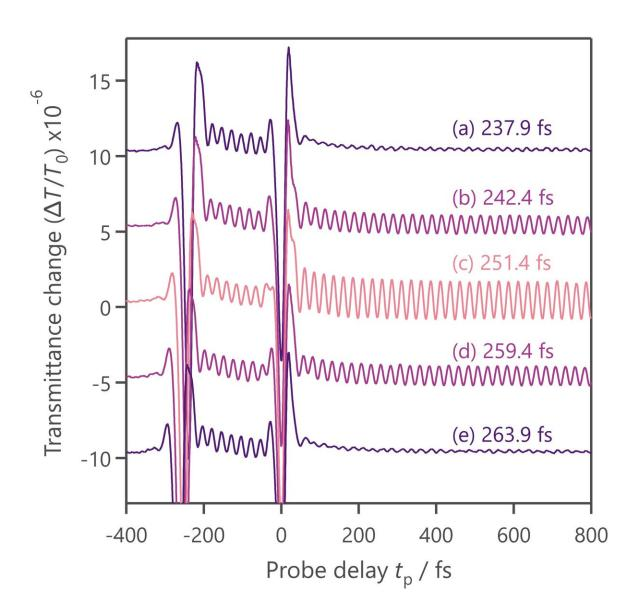
Transmittance change of the probe pulse plotted against the delay of the probe pulse with respect to the second pump pulse for five different time gaps between
