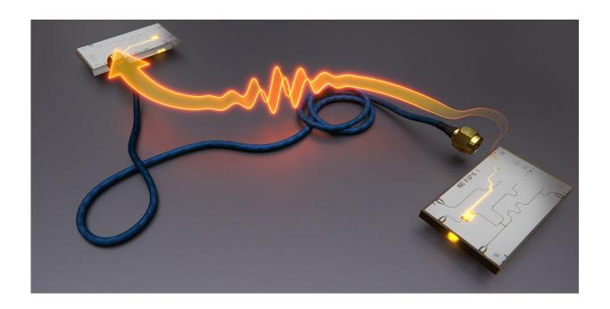
For the first time, the quantum state of a superconducting qubit was transferred with a coaxial cable to another qubit. Credit: ETH Zurich /M. Pechal, T. Walter, P. Kurpiers
