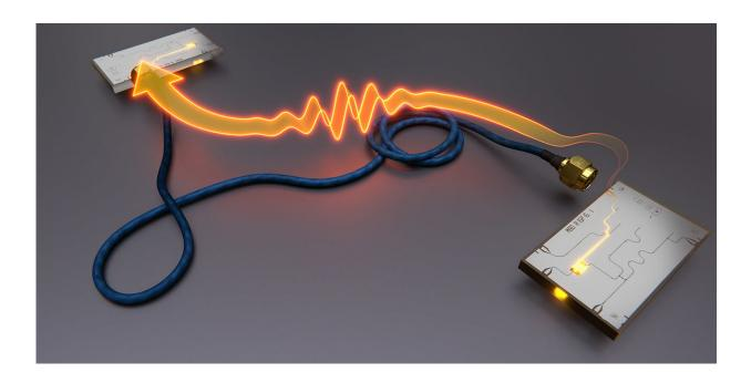
For the first time, the quantum state of a superconducting qubit was transferred with a coaxial cable to another qubit. Credit: ETH Zurich /M. Pechal, T. Walter, P. Kurpiers
