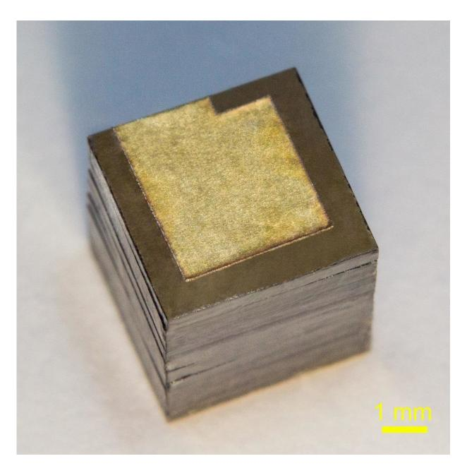
Photo of a prototype nuclear battery. Credit: Technological Institute for Superhard and Novel Carbon Materials
