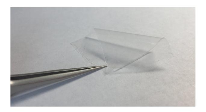
A solid polymer electrolyte film that's being utilized in lithium batteries in the research being led by Dr. Yu Zhu. Credit: University of Akron
