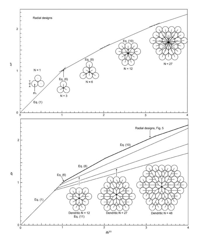
Examples of small radial distribution architectures and their efficiencies (top) versus tree-shaped or dendritic architectures (bottom) Credit: Adrian Bejan,
